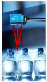
Minneapolis-based SICK, uses two independent receiver arrays mounted on both sides of a high-power, red LED and unique evaluation software to ensure continuous detection when diffused light is misdirected from bundled surfaces such as bottles, and other difficult targets. This sensor eliminates the obtrusiveness and space management issues of transitional solutions, resulting in simpler, more efficient machine designs.
